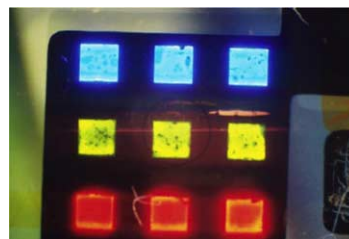
Fig. 4. An image of a simple array of 1\text{ mm}^2 polymer pixels emitting either red, green or blue electroluminescence.
